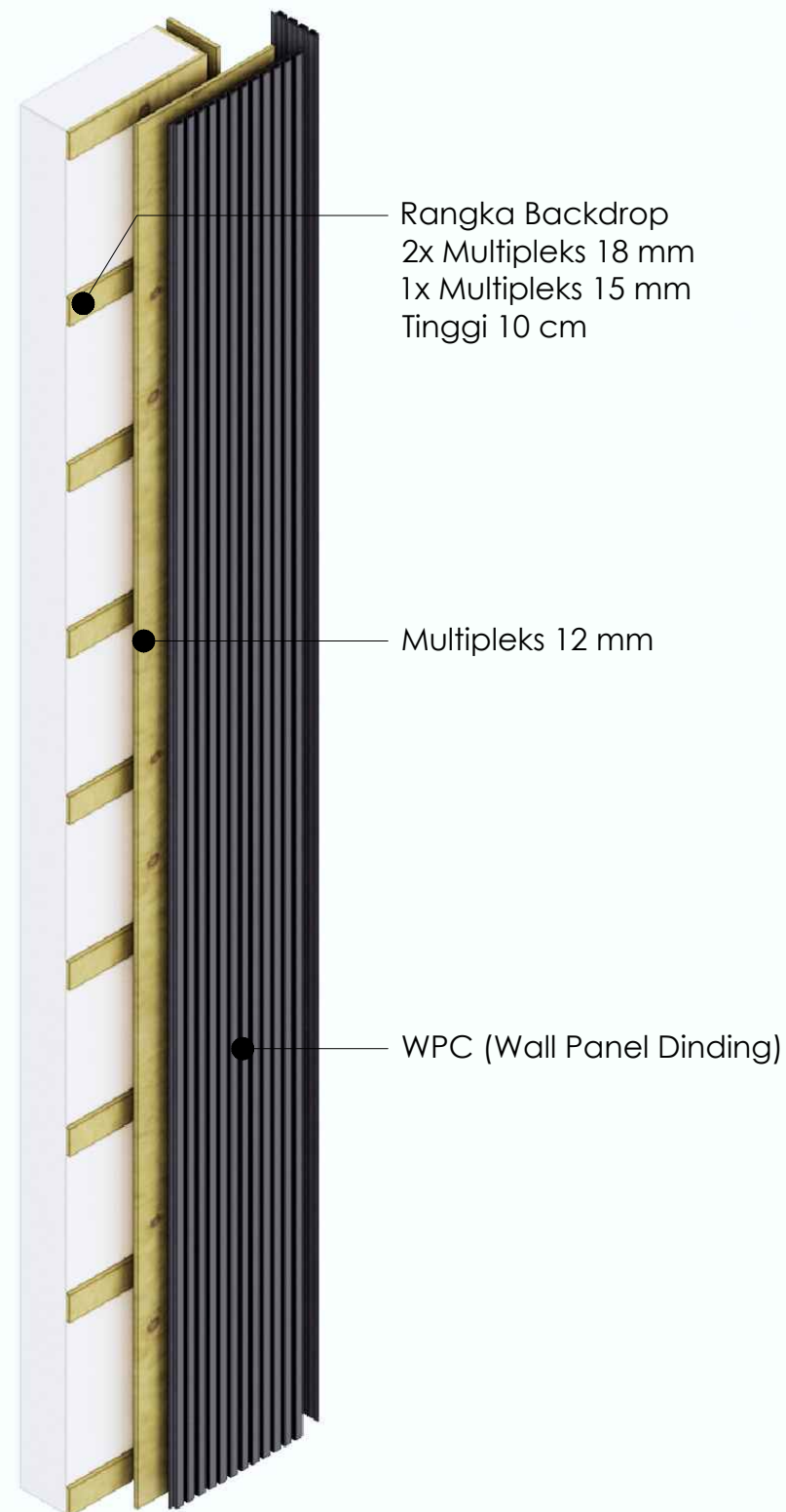
Gambar Detail: ISOMETRI KOLOM PANEL (KP-01) Non Skala
